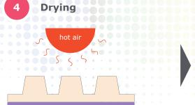
Dry the plate in a hot-air dryer after taking-off the surface water with a compressed air gun. Drying time depends on the type of the plate.
